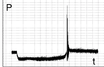
Ordinary diaphragm valve shut-off diagram – EXCESSIVE WATERHAMMER
